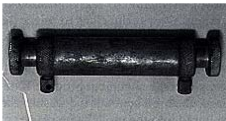
Figure 2. Internal alignment fixtures are not available in pediatric sizes and are difficult to place precisely-particularly deep within pediatric negative impressions.
