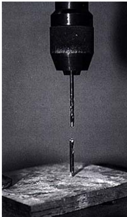
Figure 4. This simple fixture consists of a perpendicular steel pin clamped to the drill press in alignment with the drill bit.
